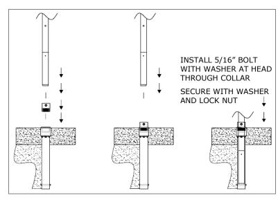
**WARNING:** The 5/16" bolt must not stick out from the lock nut and create a safety hazard.
