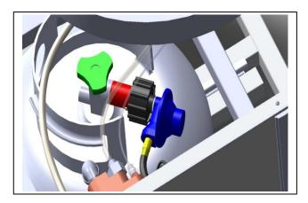
You can now connect your LP gas tank to the Fire Pit, using the standard propane gas hose with built in regulator (shown in blue). Hand tighten the propane tank gas connector (shown in black), to the tank valve (shown in red). CAUTION: Do NOT use tools to tighten this connection. Open the gas valve on the tank by turning the gas valve knob (shown in green) counter-clockwise (to the left) until fully open. See diagram located at bottom of page 5.
