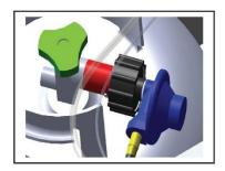
First turn the LP Gas tank (if installed) fully off by rotating the valve completely to the left until closed. Then disconnect the LP Gas tank hose with built in regulator (shown in blue) by turning the large connector (shown in black) fully counter-clockwise until the hose is completely disconnected.
