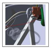
Remove the LP Gas tank hose from the gas valve (shown in bronze) at the elbow (or straight connector) coming out of the gas valve as shown above. Connect your inlet supply line, including pressure regulator to this location. Follow all local codes. Do not install without a regulator, which will limit your fuel supply to 5 inches of water column.
