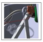
Remove the LP Gas tank hose from the gas valve at the elbow (or straight connector) coming out of the gas valve as shown above. Connect your inlet supply line, including pressure regulator to this location. Follow all local codes. Do not install without a regulator, which will limit your fuel supply to 5 inches of water column.
